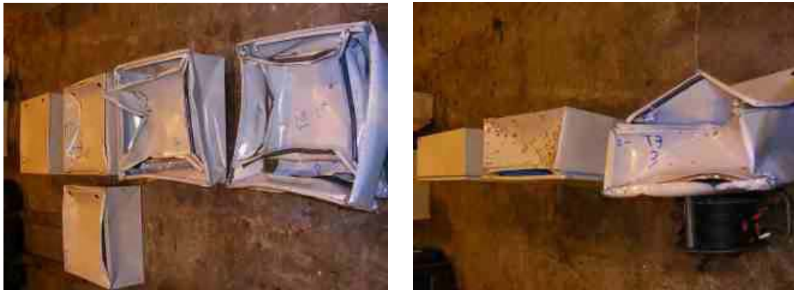
Figure B.13 The final shape of 600 mm by 600 mm by 250 mm switch boxes exposed to overpressures from 100 kPa to 960 kPa peak side-on pressure (low pressure on left and high pressure on right in the picture). The left picture shows the deformation of the front panel which faced the explosive charge. The right picture shows the deformation of the side panel which faced the explosive charge.
