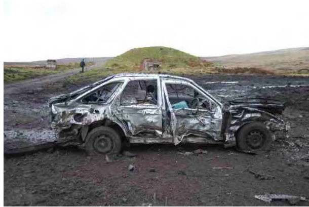
Figure B.25 Picture of a car (side oriented) exposed to a side-on overpressure of 500 kPa. Panels were deformed, but there was no significant damage to underlying supporting structure.
