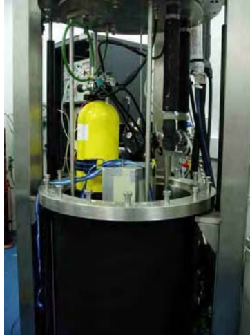
Figure B.2 A diving equipment test chamber used for hydraulic testing of switch boxes. The grey box in the centre of the chamber is the switch box. The yellow gas cylinder provides the pressure source.
