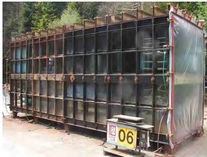
Figure B.3 The medium scale gas explosion test rig operated by GexCon, Norway.
