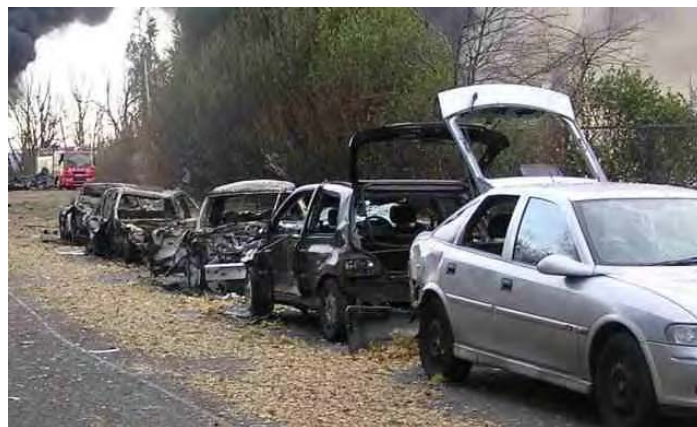
Figure B.27 A line of parked cars shows high level of damage at the far end and relatively low level at the front.
