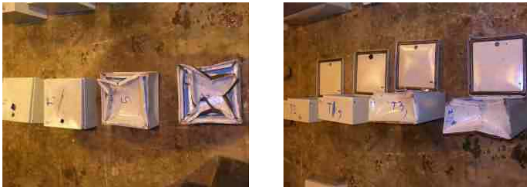
Figure B.14 The final shape of 300 mm by 300 mm by 150 mm switch boxes exposed to overpressures from 100 kPa to 960 kPa peak side-on pressure (low pressure on left and high pressure on right in the picture). The left picture shows the deformation of the
