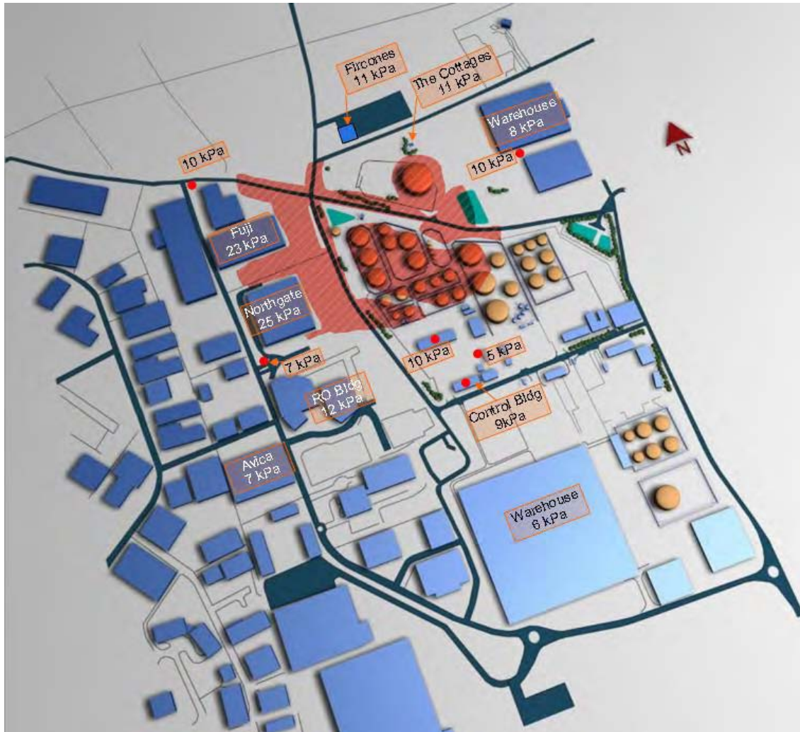
Figure 11 Overpressure indicators (the area where damage suggests overpressures > 200 kPa is shown shaded)
