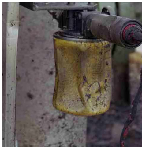
Figure B.17 A crushed oil filter in Buncefield.
