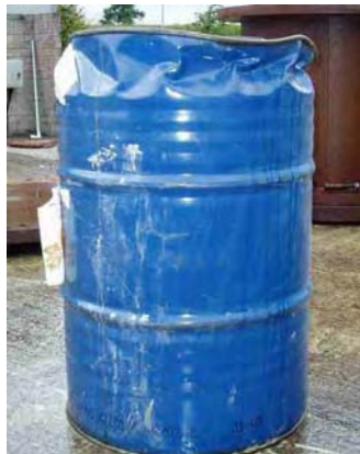
Figure B.7 Fully plastic longitudinal sidewall buckling in the ullage. This was observed at above 200 kPa but less than 300 kPa.
