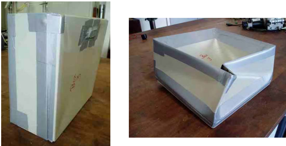
Figure B.16 Views of damage to box caused by application of 400 kPa overpressure – over a period of around 2 seconds. Large deformation of back and side – tearing of weld between back and sides. Some plastic deformation of front (final volume to initial volume ratio of 50%).
