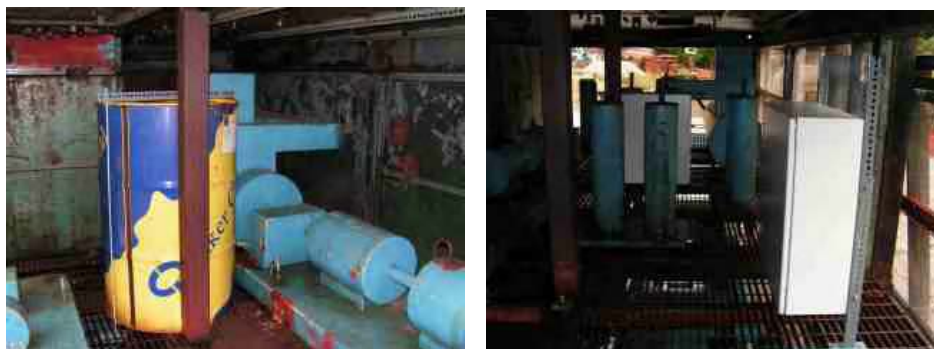
Figure B.4 Test objects exposed to explosion overpressure loads: an empty oil drum (left) and two switch boxes at different locations (right)
