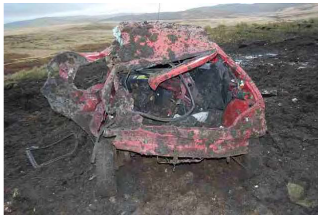
Figure B.26 Picture of the end view of the Peugeot car (rear oriented) after exposed to blast overpressure. Severe damage occurred to both panels and underlying structures.
