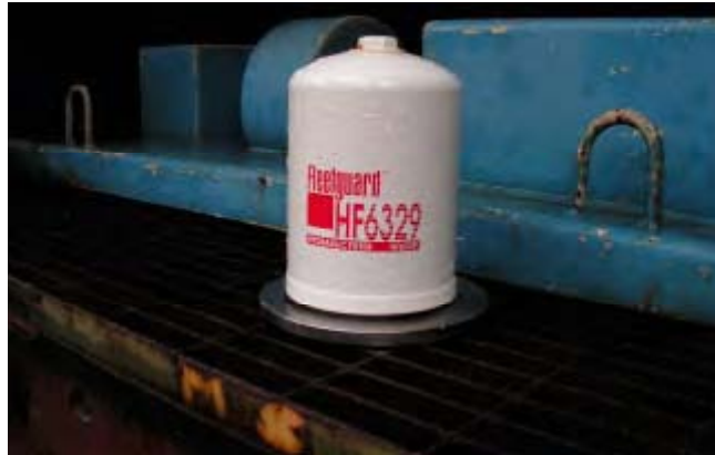
Figure B.18 An oil filter which had been exposed to an gas explosion test of 180 kPa was not damage.
