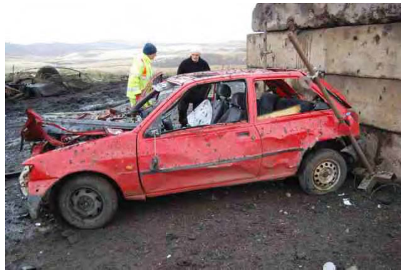
Figure B.24 Picture of a car (nose oriented) after exposed to blast overpressure. Panels were deformed, but there was no significant structure deformation on this side of the car.
