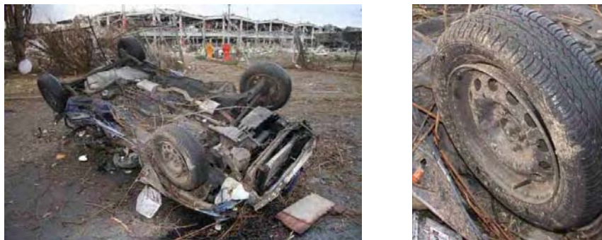
Figure B.19 Car tyre pushed off the rim during the explosion.
