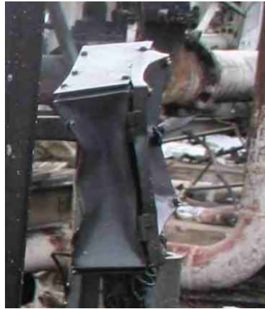
Figure B.10 A crushed junction box, close to the northern edge of the HOSL site.
