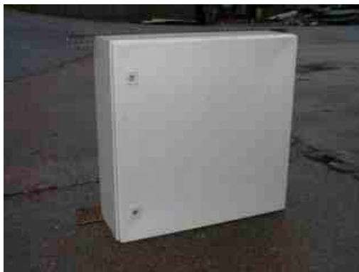
Figure B.11 View of the only switch box which had been deformed in the gas explosion test.
