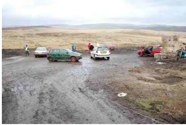
Figure B.23 Arrangement of cars before the test explosion. There were 5 cars arranged at various distance to the explosive charge which was located between the white car near the centre of the picture and the red car at a distance behind it.
