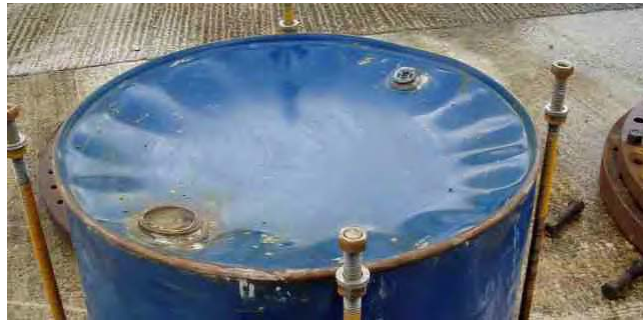
Figure B.8 Plastic deformation of drum end cap: (left) a drum in Buncefield and (right) after a static pressure test at 200 kPa.
