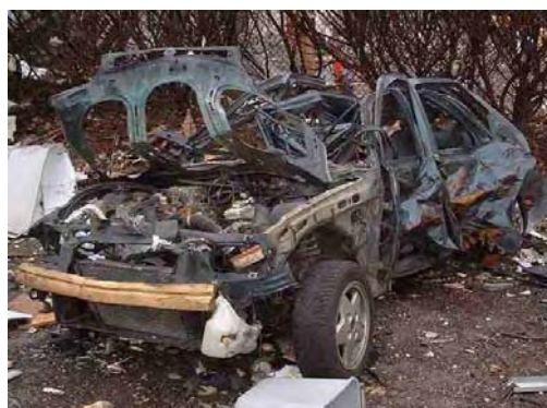
Figure B.21 Typical car damage, with rear tyre blown off inner rim.
