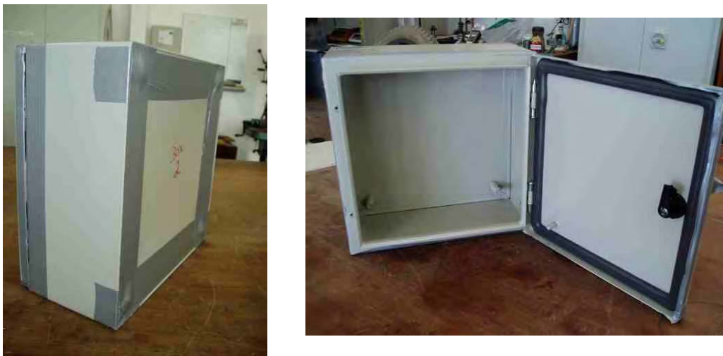
Figure B.15 Two views of damage to the 300 mm by 300 mm switch box by 100 kPa overpressure: slight bowing of back but no plastic deformation of the front panel.
